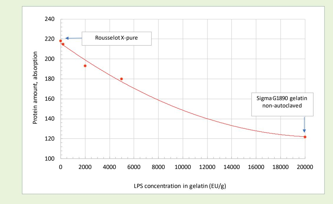
The cellular activity and growth of the endothelial cell line was largely influenced by endotoxin. The G1890 Sigma gelatin with endotoxin level of 2000EU/g gave significantly lower cellular activity compared to purified Rousselot X-pure gelatin with endotoxin level <10EU/g.
