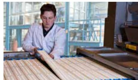
*Gummies are deposited in flexible silicon molds. The absence of starch makes the process completely clean. ▶*
